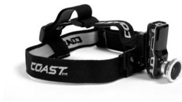
Figure 1: Our light-weight, low-cost head-mounted camera with fisheye lens.
